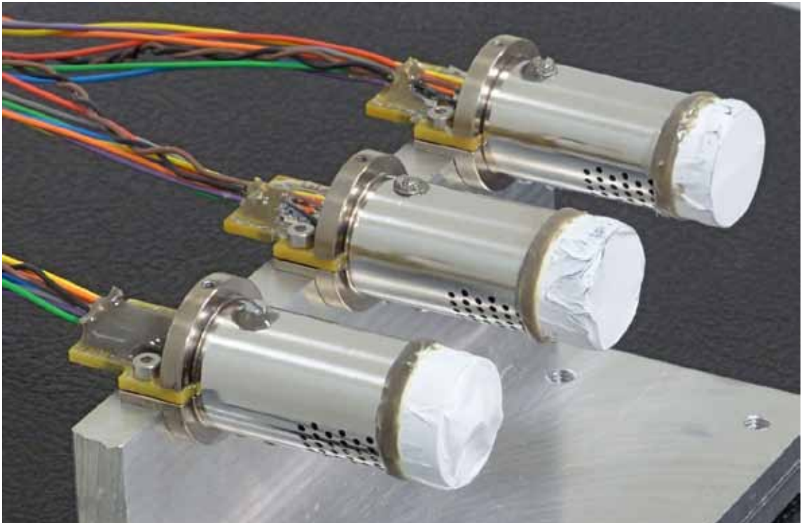
Figure 3.3. DREAMS-H, a humidity device for ExoMars 2016, is assembled in the Finnish Meteorological Institute. Corresponding instrument is currently operating on Mars on board of the Mars Science Laboratory. photo: Markku Mäkelä, Finnish Meteorological Institute
