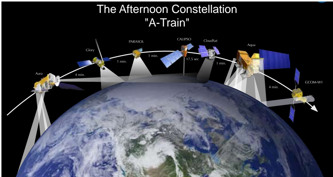
Figure 5.10. International A-Train constellation consists of seven international Earth Science satellites that fly within approximately ten minutes of each other to enable concurrent science.
