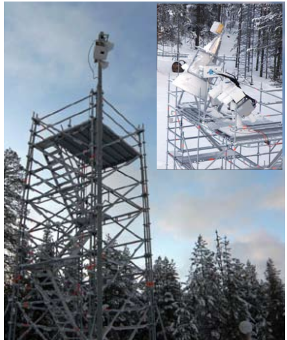
Figure 5.15: Reference instruments for ESA CoReH2O SAR, ESA SMOS and NASA/Jaxa AMSR-E at Sodankylä.
