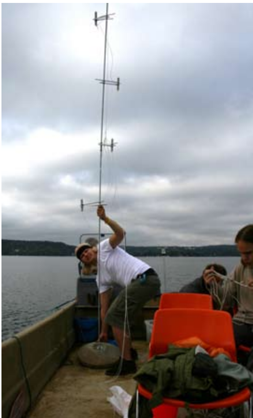
Figure 5.18. A series of optical sensors are deployed for a vertical profile of light level.
