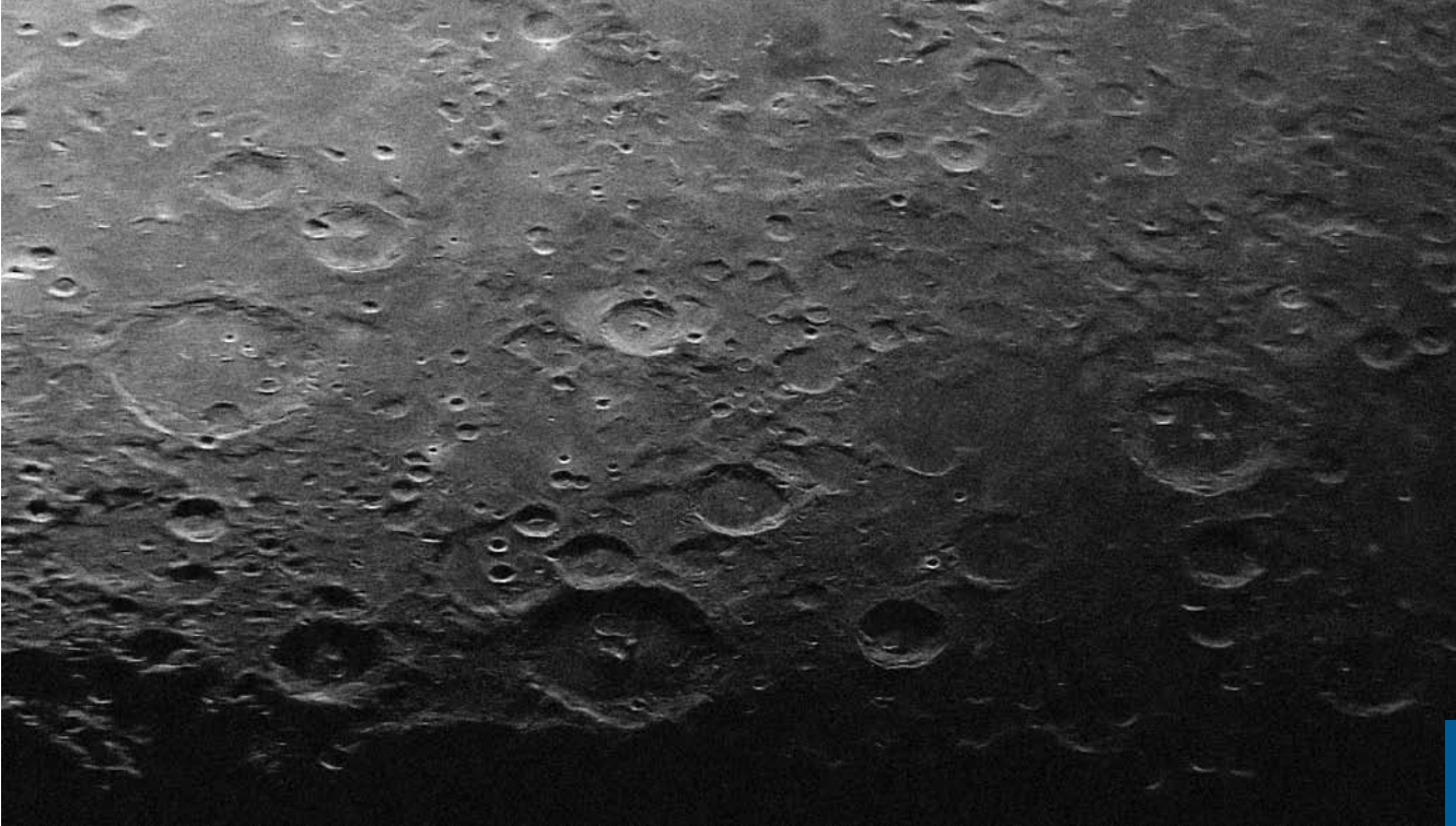
Figure 4.8. An unfocused delay-Doppler image of the Lunar surface obtained with the EISCAT UHF system. The range resolution is approximately 600 m. Because the image is unfocused, Doppler smearing can be seen on the edges.
