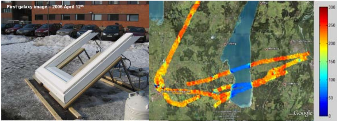
Figure 5.29. HUT-2D remotes sensing radiometer developed by RAD/STG. The instrument is pointed upwards for Galactic measurements. Nominally, the instrument is attached at the bottom of the fuselage of the research aircraft Skyvan. Right: Brightness temperature images composed using measurements of HUT-2D instrument from several overpasses of a test area near Munich during the SMOS validation campaign in 2008.
