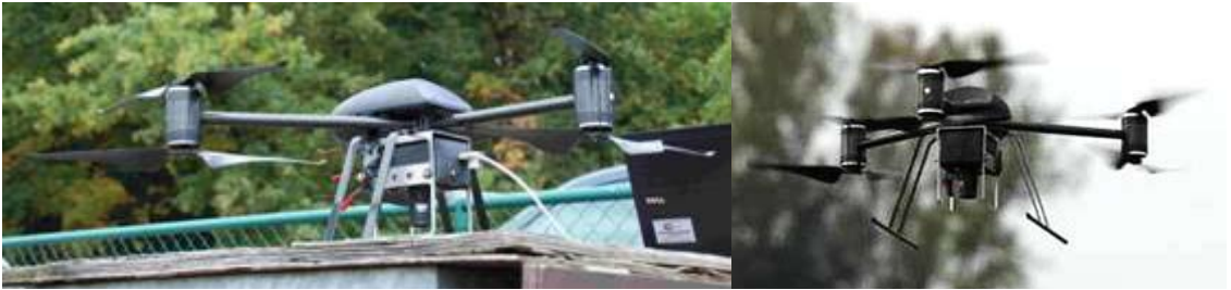
Figure 5.35 VTT Staring FPI Hyperspectral Imager integrated on VITO six-rotor rotorcraft.
