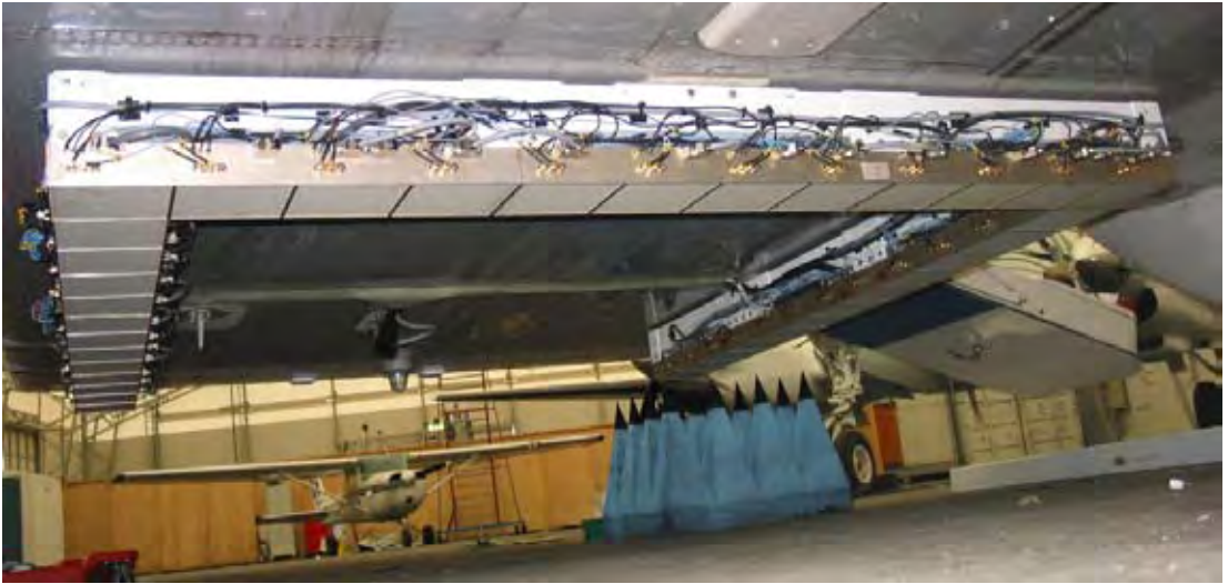
Figure 5.21. HUT-2D radiometer mounted underneath the TKK research aircraft fuselage.
