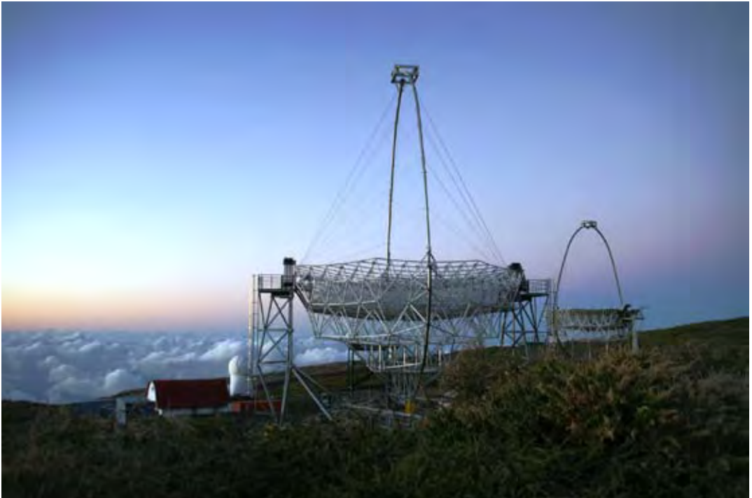
Kuva 4.30. The MAGIC TeV telescope on La Palma, Canary Islands. MAGIC II, under construction, is in the forefront.
