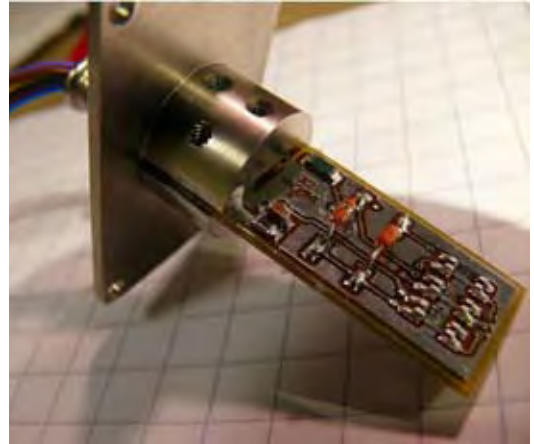
Figure 4.10. Conceptual drawing and a test unit of the DigiHUM instrument developed for the Mars Science Laboratory.
