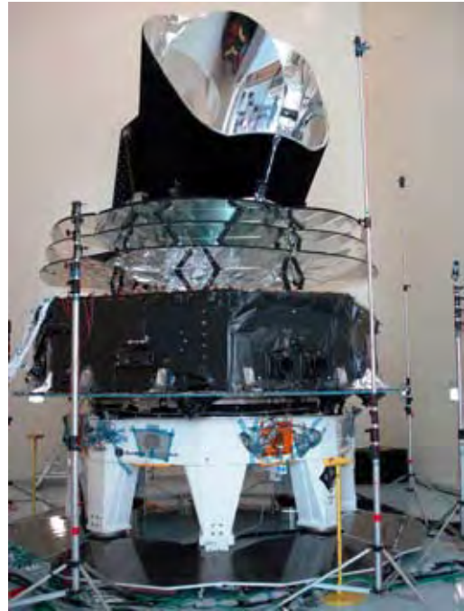
Figure 4.23. The Planck satellite in acoustic tests (courtesy of Thales Alenia Space and ESA)
