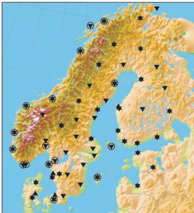
Figure 5.1. Nordic Geodetic Observing System (NGOS) network connect existing space geodetic and traditional networks. Upside-down triangles denote permanent GPS stations, triangles absolute gravity points, and circles are tide gauges planned for the NGOS network.
