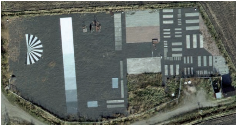
Figure 5.5. The Sjökölla test field, test targets for the spatial resolution and radiometry.
