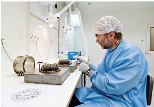
Figure 4.1. Preparation of a set of pressure and humidity sensors of Vaisala Oyj for space qualification tests in the new space technology laboratory of the FMI.
