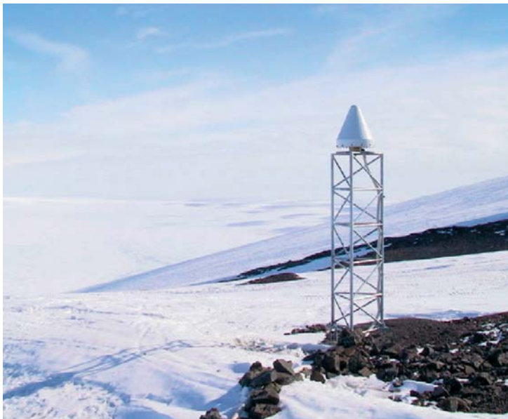
Figure 5.2. Antenna mast of the Finnish Antarctic permanent GPS station. (Photo H. Koivula)
