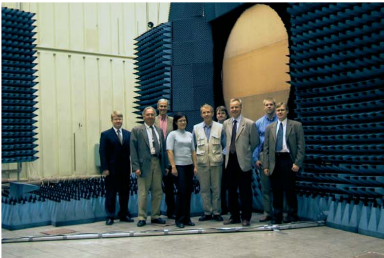
Figure 4.24. A 3 m submillimetre wave hologram developed for 1.5 m diameter ADMIRALS Representative Test Object (RTO) telescope tests at 322 GHz. The same method is planned to be used for testing the Planck Telescope. In the photograph, ESA representatives and the research group are also shown.
