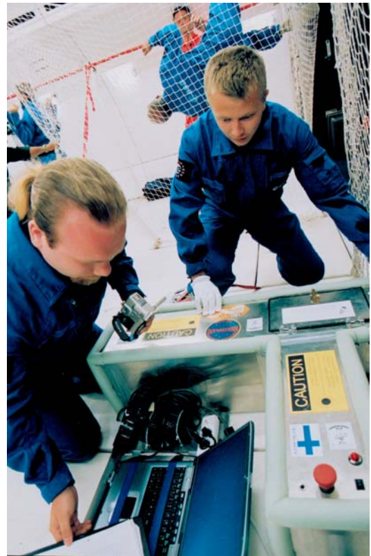
Figure 4.9. Jyri Näränen and Seppo Heikkilä measuring light backscattering from Lunar analogue material in microgravity.
