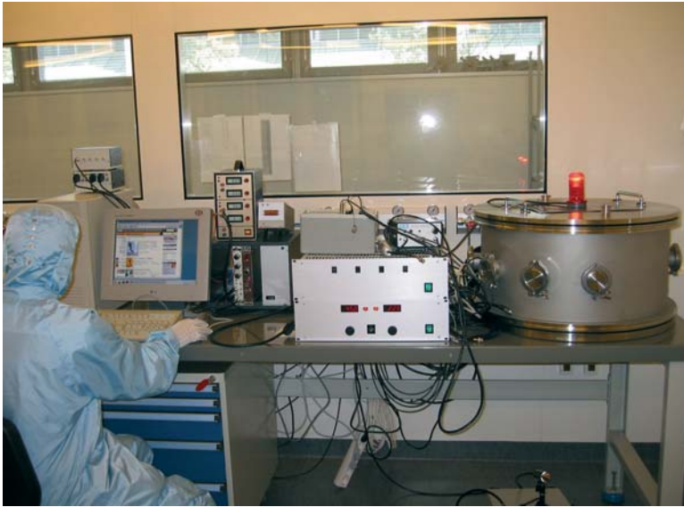
Figure 4.19. Testing of the Solar X-ray Monitor of the SMART-1 spacecraft in the newly-established clean room at UH/PHYS.
