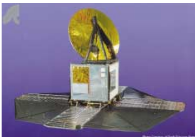
Figure 3.6. 119 GHz receiver developed by Ylinen Oy for ODIN satellite.
