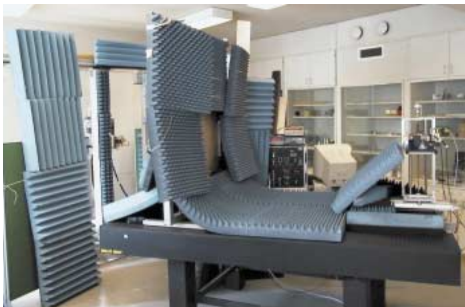
Figure 4.11. Measurement set-up for testing the quiet-zone field of the 60 cm hologram at 310 GHz.
