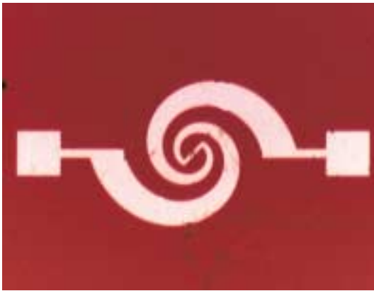
Figure 3.4. An antenna-coupled microbolometer. The antenna is sensitive to frequencies between 200 GHz up to 1 THz. Radiation power absorbed in this band heats up a microscopic niobium thermometer strip, located at the feed of the spiral antenna. Prime Metorex International.
